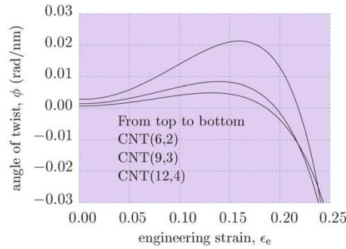
Fig. 2. Extension-induced twist versus axial engineering strain.
