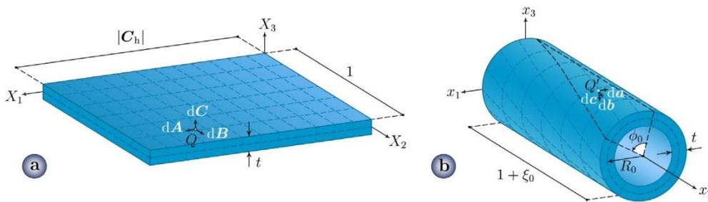
Fig. 1. Geometry of (a) unit strip of graphene (lamina), and (b) the obtained SWCNT (elastica).
