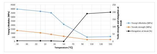
Figure 1. Temperature dependence of mechanical strength.
