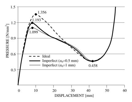
Fig. 2. Fundamental load-displacement path for apex node
