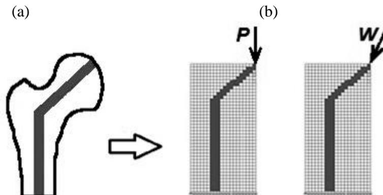
Fig. 1. Hip joint endoprosthesis (a) and computational model (b).
