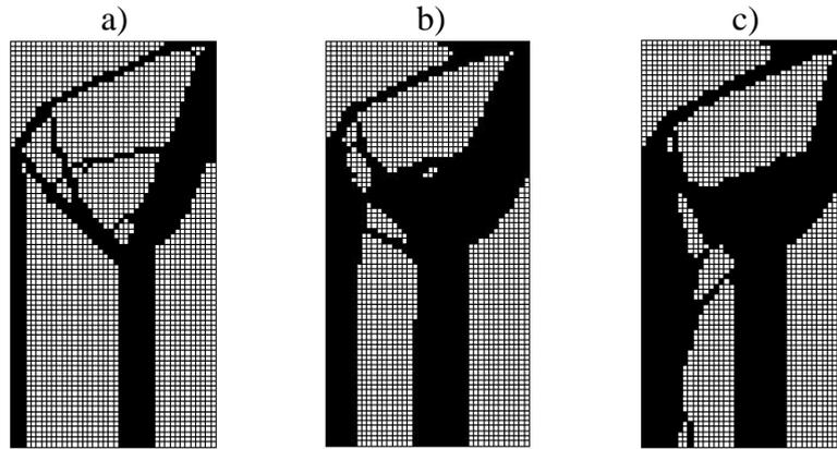
Fig.2. 0/1 topologies for  $P$  loading – for  $\alpha = 0,3$  a)  $\alpha = 0,5$  b) and for  $W$  loading - for  $\alpha = 0,5$  c)
