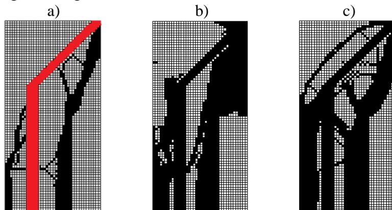
Fig.3. 0/1 topologies with implant for  $P$  loading – for  $\alpha = 0,3$  a)  $\alpha = 0,5$  b) and for  $W$  loading - for  $\alpha = 0,5$  c).
