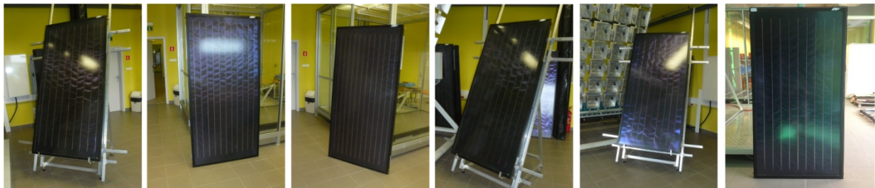
Figure 3. Test samples of a solar collector with various geometrical parameters.
