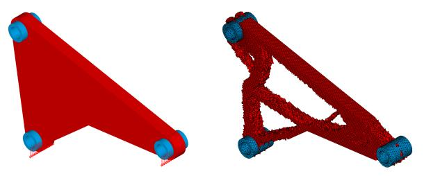
Figure 1. Initial structure (left), obtained topology (right)
