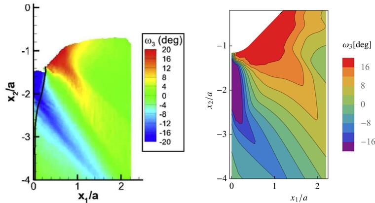
**Figure 1.** Wedge indentation in Ni single crystal: experimental results [4] (left) and numerical results calculated using the rate-independent model,  $n = 20$  (right).
