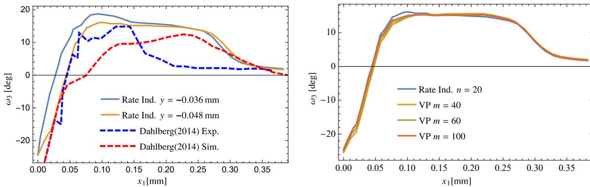
**Figure 2.** Comparison of the obtained lattice rotations with experimental and numerical results from [4].
