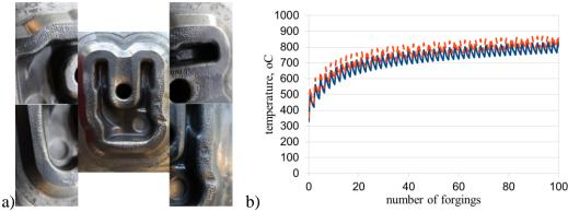
Fig. 1. View of dies for forging of the fork after 6000 of forgings (a) and changes of the die temperature during forging (b) – dashed line for a new die and solid line for a worn die.
