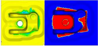
Fig. 2. The die wear measured using scanner (left) and calculated by the model (right).
