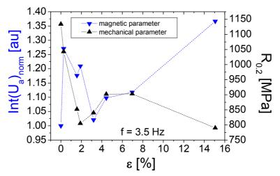
Fig. 2. Variations of the integral calculated from MAE envelopes and yield point versus creep prestrain
