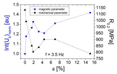
Fig. 1. Variations of the integral calculated from MBE envelopes and yield point versus creep prestrain [5]
